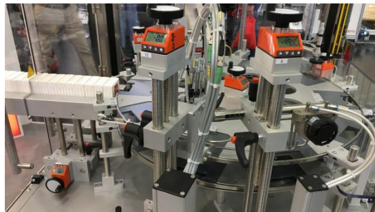
Elesa DD52R-E-RF electronic position indicators application on a JW Verpackungstechnik packaging machine
